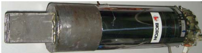
Fig 11: (Left) Bicorn made PMT with a lead shield around the NaI scintillator and a collimator (10° x 10°). (Right) The model of the shield and collimator for GEANT4 simulations.
