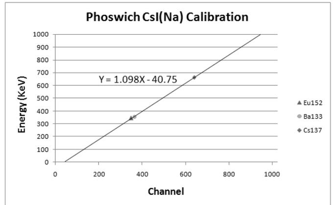
**Figure: Channel-Energy calibration curve for NaI(Tl) crystal of Phoswich detector**
