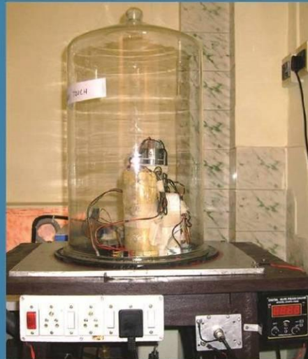
Dynamic Cosmic Ray Spectrum for D74 Mission with raw data and processed data (Left). Setup for vacuum test of payloads (Middle). A typical X-Ray scintillation detector payload for balloon missions (Right).
