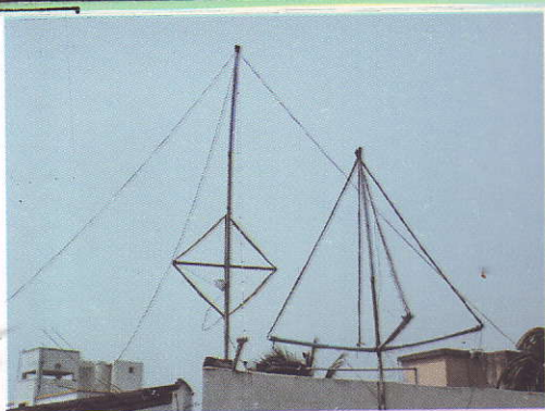
Different types of antennas (from L to R) in regular data acquisition such as loops and cross loops, under sea and for balloon flights which are used at ICSP.
